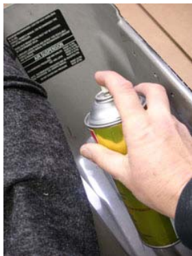
Before spraying, mask the lip of the box for overspray. Spray adhesive on the floor, one end and one side.
