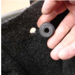
Position Lining in Bag and reinstall grommets. These act as locator pins to position lining into place.
