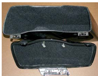
Allow bags and lids 1/2 hour to completely dry. They are now ready to reinstall hinge and put back on your bike.
